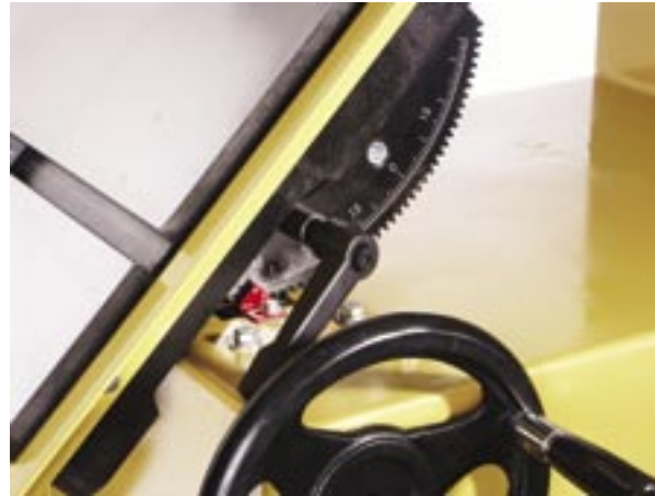
New Crank handle tilts Table 45° right and 10° left
