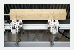
Without magazine operation (only as insertion device) rectangular blocks of wood of up to 200 mm can be inserted.
