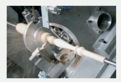
The belt grinding unit on 4<sup>th</sup> axis with PC switching, pointed and flat grinders for round profiles.
