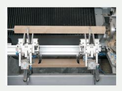
The magazine / inserting device centres rectangular blocks of wood of 20 up to 120 mm and a length of 100 up to 1800 mm automatically without adjustment.
